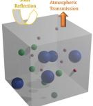
Draft of a radiative cooling composite material: a combination of resonant nanoparticles engineered to reflect solar light with precision, simultaneously facilitating efficient heat radiation through the atmospheric window.
